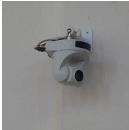
Wall mounted Sony EVI-D70 remote camera for clear projection and recording of images with preset or full PTZ joystick control
