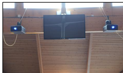
Dual Eiki X85 Projectors, 60" relay plasma and remote camera
